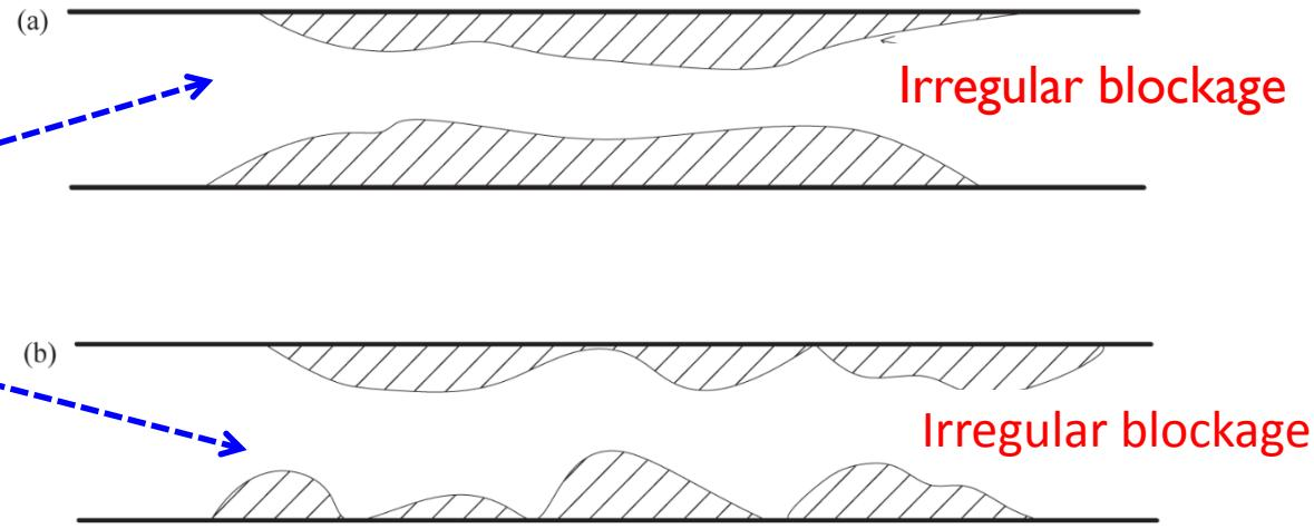
**Fig. 1** Sketches of irregular blockages in practical water pipelines
